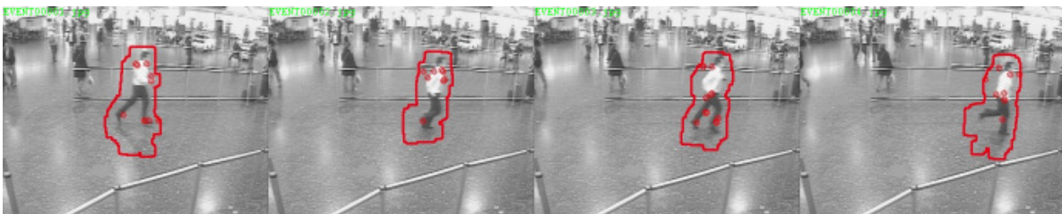
Figure 3: Action detection for PersonRuns based on a blob from a change detection.
