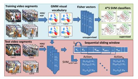
Figure 4: Block diagram of the surveillance event detection system.
