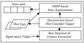
Figure 1: Overall system components
