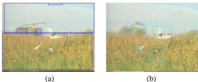
Figure 3: Example region segmentation results (bounding boxes of extracted regions): (a) background segmentation, (b) foreground object segmentation.
