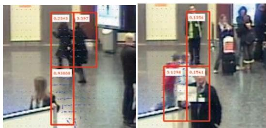
Figure 3: Examples of simultaneous events that are close to each other and therefore detected as a single event.
