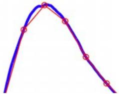
For the Intersection Kernel  $h_i$  is piecewise linear, and quite smooth, **blue plot**. We can *approximate* with fewer uniformly spaced segments, **red plot**. Saves time & space!
