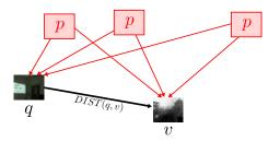
• Let  $S = \{p_1, ..., p_m\}$  be a set of pivots, then:  $DIST(q, v) \ge \max_{p \in S} \{|DIST(p, q) - DIST(p, v)|\}$
