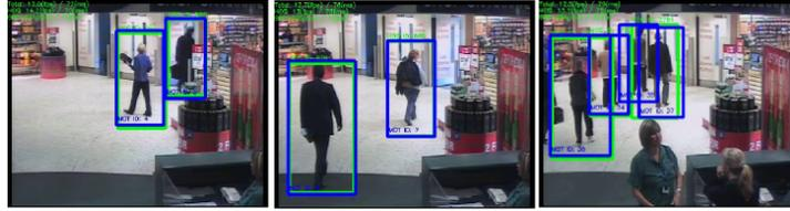
Figure 3: Examples of person detection and tracking: (green) HOG detections, (blue) tracked detections
