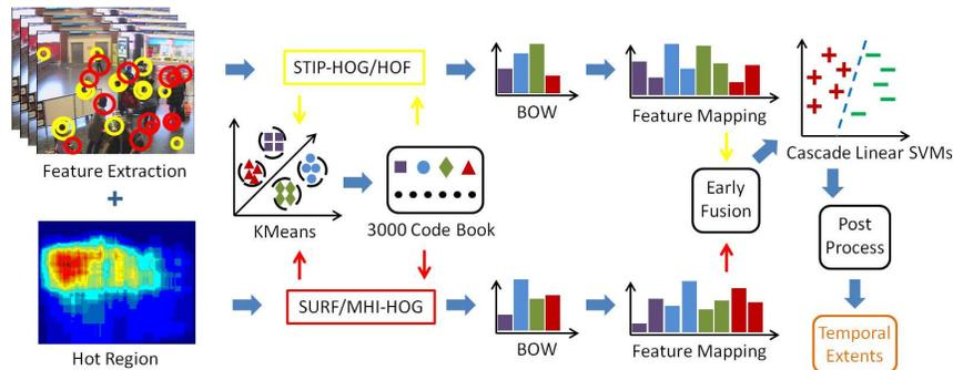
Figure 1: MediaCCNY surveillance event detection system architecture.
