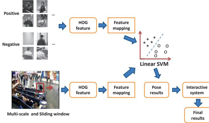
Figure 2: Key pose based interactive event detection system architecture.
