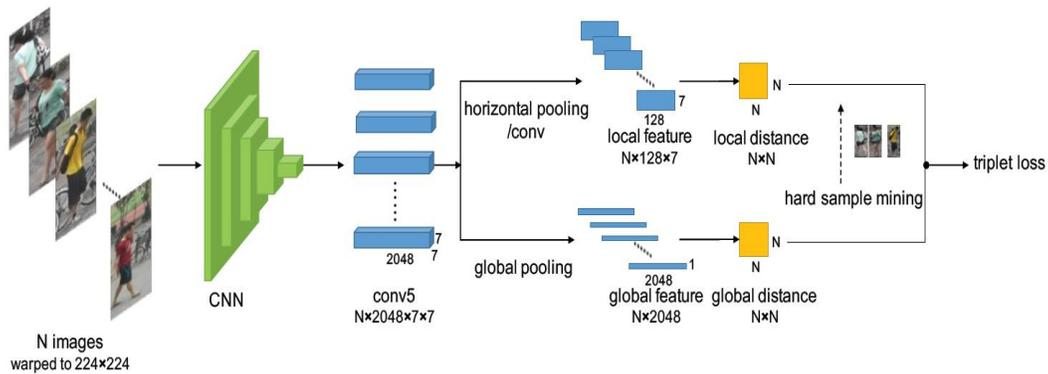
Figure 4: The framework of AlignedReID. Both the global branch and the local branch share the same convolution network to extract the feature map. The global feature is extracted by applying global pooling directly on the feature map. For the local branch, one  $1*1$  convolution layer is applied after horizontal pooling, which is a global pooling with a horizontal orientation. Triplet hard loss is applied, which selects triplet samples by hard sample mining according to global distances.
