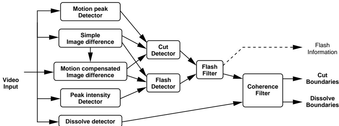
Figure 1: Shot boundary detection system architecture
