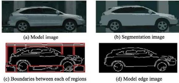
**Figure 11 Generation of the model edge image.**
