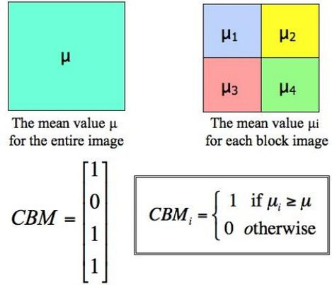
Figure 8. Example of CBM for  $2 \times 2$  block images.
