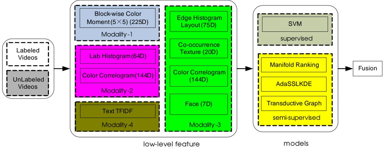
**Fig. 1.** The MSRA TRECVID 2006 Feature Extraction pipeline
