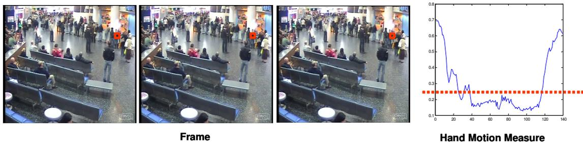
**Figure 9.** Hand motion is detected in a region (shown as red rectangle) and is plotted on the right. Red line shows the threshold used to find the range of frames with no hand motion.
