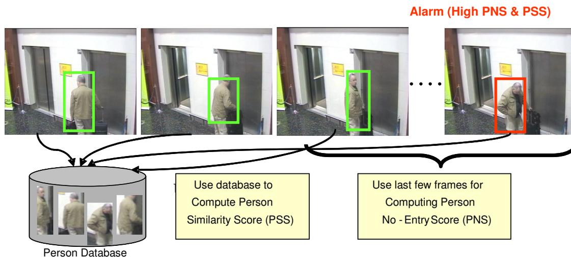
Figure 3: Algorithm for "Elevator Non Entry" event detection.
