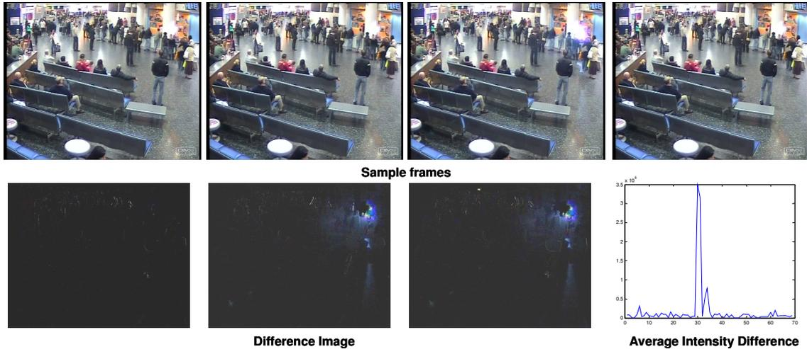
**Figure 8.** Sample frames (top row) and the difference between consecutive frames (bottom row), e.g., the first difference image corresponds to the difference between the first and second frames. The third frame contains flash event. The plot on bottom right shows the sharp change in pixel intensity on flash event.
