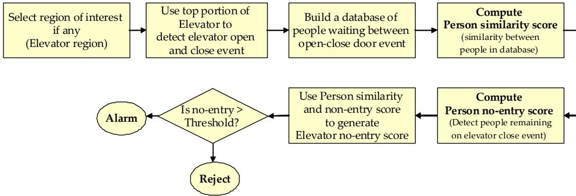
Figure 4. Basic steps of Elevator No Entry Event detection algorithm.
