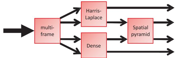
**Figure 3:** General scheme for spatio-temporal sampling of image regions, including temporal multi-frame selection, Harris-Laplace and dense point selection, and a spatial pyramid. Detail of Figure 2, using the conventions of Figure 1.
